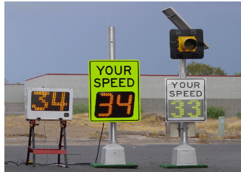
Figure 1 - from left to right: RU2 FAST 250, IDC VSC-1520 and 3M 1VL Driver Feedback display. Test conditions: moderately overcast, 4-6 p.m. in August; viewed approx 35 ft away; 10 ft off center of IDC unit. All units face west.
