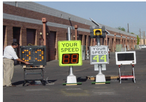
Figure 2 - left to right: PSC Traffic Monitor Speed Display; IDC VSC-1520; 3M 1VL Driver Feedback and RU2 FAST 250 (blank) display. Test conditions: clear and sunny 7-9 a.m. in August; viewed approx. 40 ft away ; centered to the group. All units are facing east.
