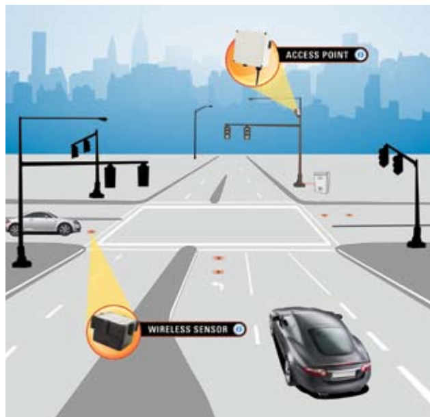
Typical Wireless Vehicle Detection System installation.
