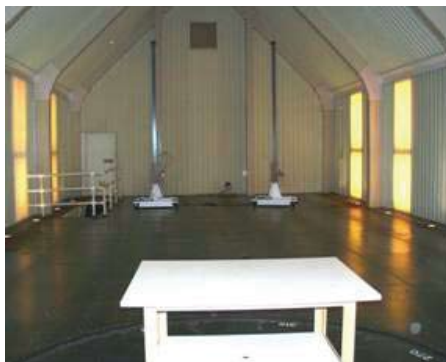
Inside photograph of an open area test site where radiated EMC testing is performed. The table on turntable where the equipment under test is placed is in the foreground with the receiving antennas in the back 10 meters away from the equipment under test. The composite of the building is all plastic, no metal. Measuring equipment is located below the metal ground plane.
