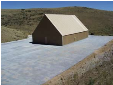
Outside photograph of an open area test site where radiated EMC testing is performed. The metal ground plane is extended outside the composite plastic building to provide for repeatable testing results.
