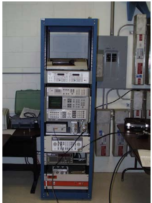
Lab Eq Anechoic Controls - Laboratory measuring equipment rack used to measure radiated and conducted emissions testing.
