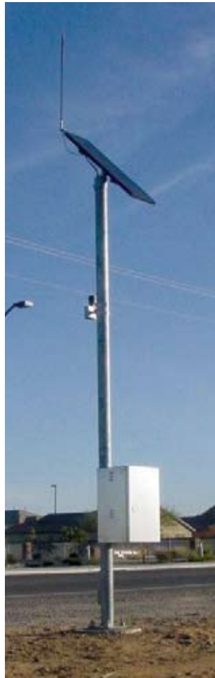
Figure 3, optical detector unit with radio transmitter located to look up the station driveway.
