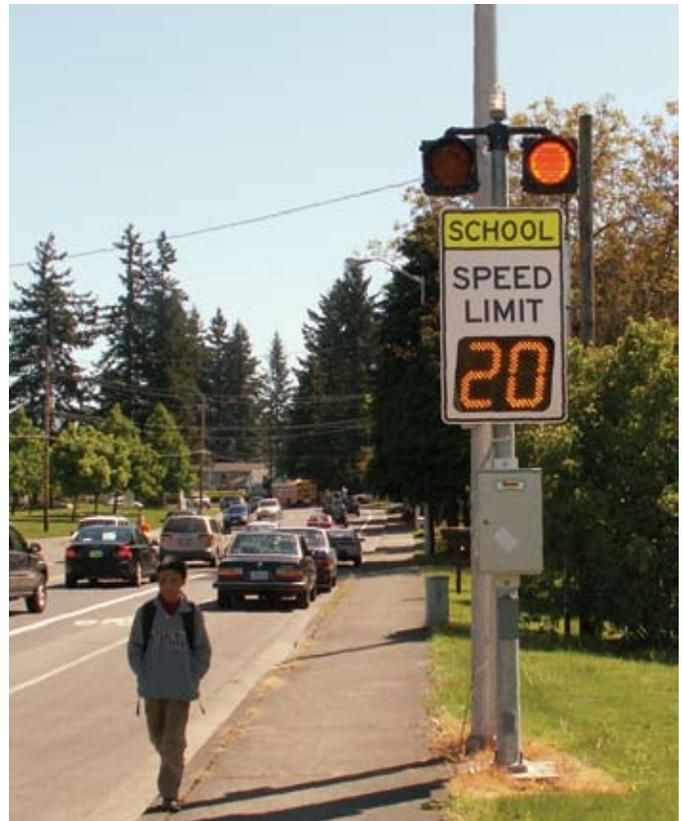
In the example above, the signs all have built-in atomic clock synchronization to assure that the signs are always exactly in sync with each other.
